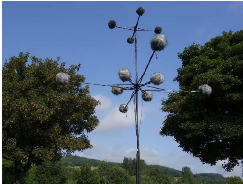
FIGURE 1 –THE 12 CHANNEL 3D MICROPHONE ARRAY DESIGN
