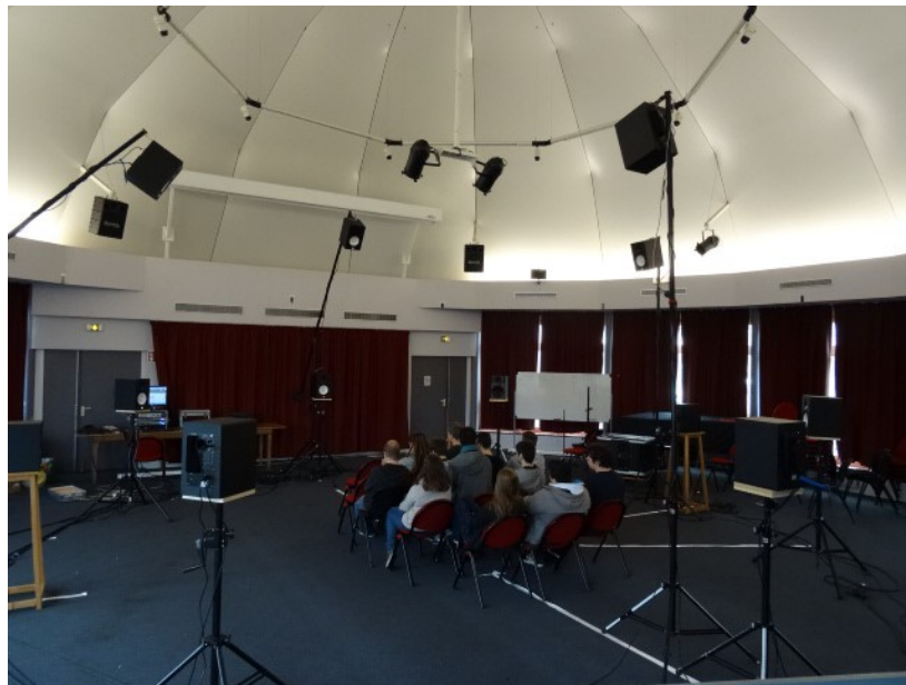
FIGURE 2 – 12 CHANNEL LOUDSPEAKER CONFIGURATION ITEMM – LE MANS, FRANCE
