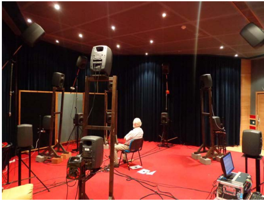
FIGURE 3 – 12 CHANNEL LOUDSPEAKER CONFIGURATIONS (NSEW AND AURO 3D) – GALAXY STUDIOS, MOL, BELGIUM
