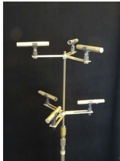
FIGURE 9 – 'HEXAPHONIE' ARRAY (ORIGINAL PHOTO BY ROGER PICARD) RADIO FRANCE
